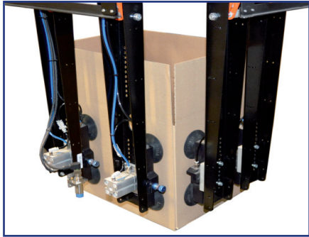
Square Case Erecting Eight vacuum powered suction cups hold the blank in the correct position after it leaves the magazine. Both leading panels are held securely.
